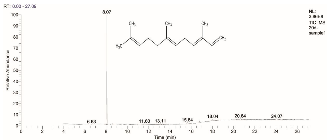
Figure S2. GC-MS total ion chromatograms of synthesis product from engineered strain expressed Fsso
